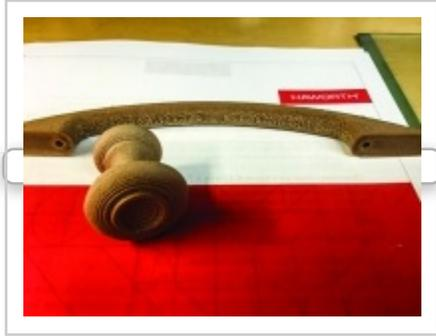
Michigan Technological University used a mixture of finely ground wood powder and plastic resin to 3-D print a door pull and handle, shown above. Researchers at the university hope to launch a \$25,000 research program with the West Michigan Zero Waste to Landfill user group to develop the technology to be able to use wood waste from the region's office furniture manufacturers.
